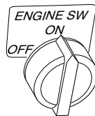
Figure 16 - Engine Switch In ON Position (All Models Except MGH5000EIE and MGH6500AIE)
